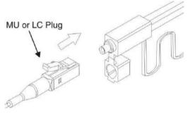
3. Push the Outer Shell to start cleaning the MU/LC connector end face. A "click" sound indicates end of cleaning process. Close the cover after use.
