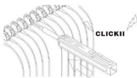
Be careful **not to slant** the One-Click Cleaner while inserting it into the adapter. **Avoid** applying excessive force during insertion, as this may cause damage to both the connector and the One-Click Cleaner MU/LC. If you encounter resistance while pushing the outer shell, remove the One-Click Cleaner from the adapter and ensure that there are no large debris particles obstructing the cleaning process.
