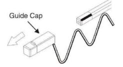
2. Insert tip of cleaner into MU/LC Adaptor
