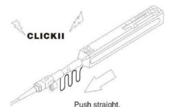
Be careful **not to slant** the MU/LC connector while inserting it into the guide cap. **Avoid applying excessive force during insertion**, as this may damage both the connector and the One-Click Cleaner MU/LC. If you encounter resistance while pushing the outer shell, remove the One-Click Cleaner MU/LC from the connector and ensure there are no large debris particles obstructing the cleaning process.
