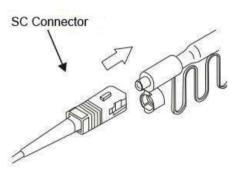
3. Push the Outer Shell to start cleaning the SC/FC/ST connector end face. A "click" sound indicates end of cleaning process. Close the cover after use.
