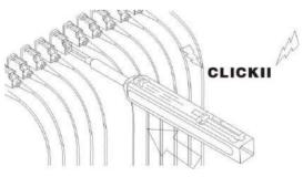
Be careful **not to slant** the One-Click Cleaner while inserting it into the adapter. **Avoid** applying excessive force during insertion, as this may cause damage to both the connector and the One-Click Cleaner SC/FC/ST. If you encounter resistance while pushing the outer shell, remove the One-Click Cleaner from the adapter and ensure that there are no large debris particles obstructing the cleaning process.
